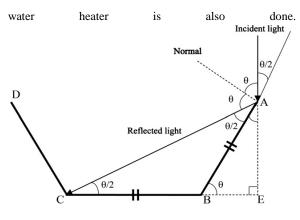
Fig.2 V- trough solar water heater
