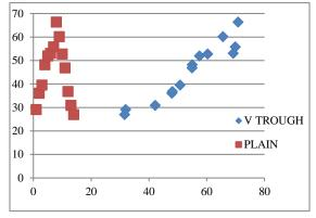
**Fig. 7** Graphical Comparison of Efficiency of Flat Plate Solar Water Heating System with V-Trough Solar Water Heating System
