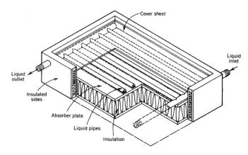
Fig.1 Flat Plate Collector
